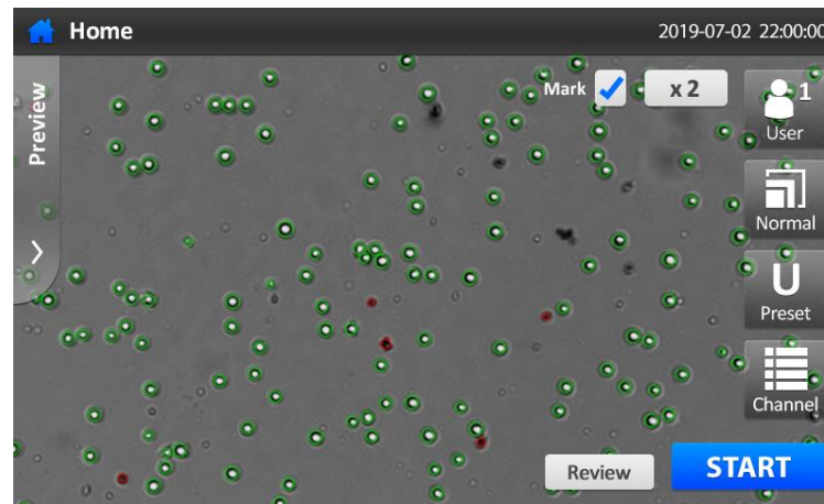
If press Mark , the detection mark is displayed according to the selected preset. Live/Dead definition can be modified at this stage.
